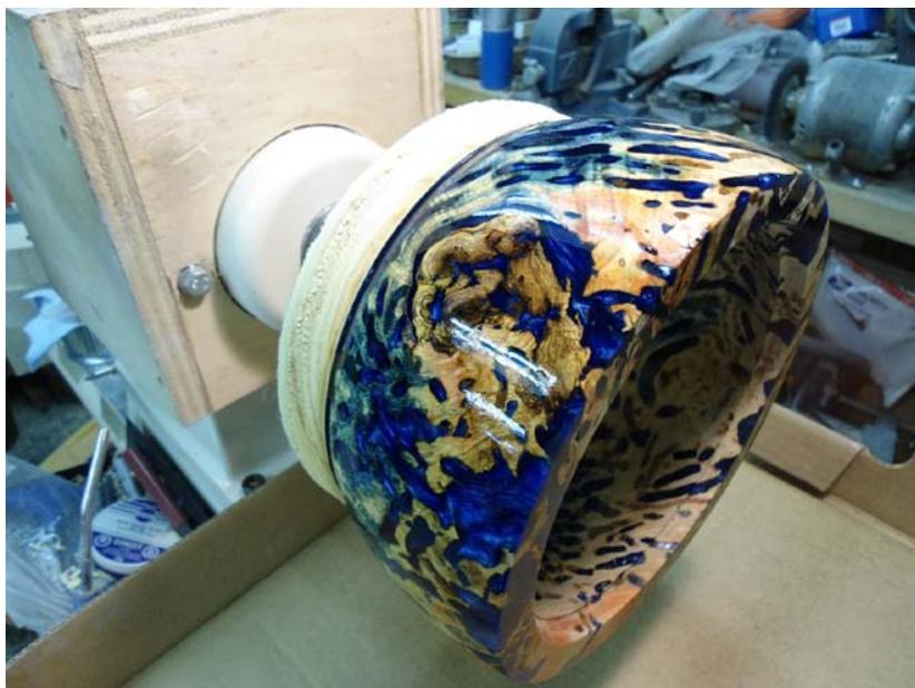
Loose Form - the core material is allowed to float or remain suspended in the casting resin. Usually requires some sort of cap to prevent overflow of the resin and material.
